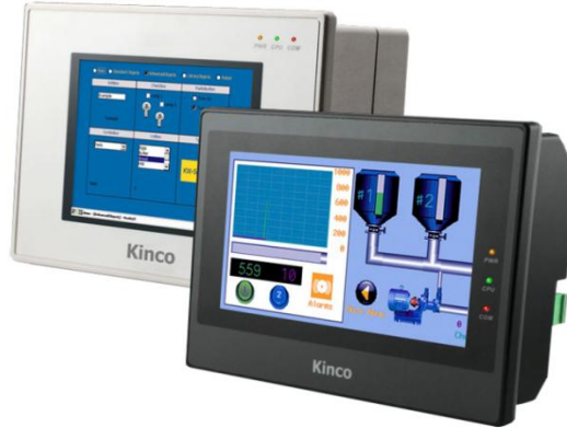
Figure 4.6 Typical HMI panel
