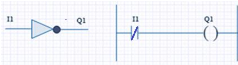
Figure 3.7: NOT Gate Symbol and Ladder Diagram
