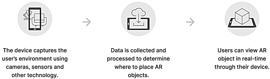
Figure no 4.10- Augmented Reality Working Principle
