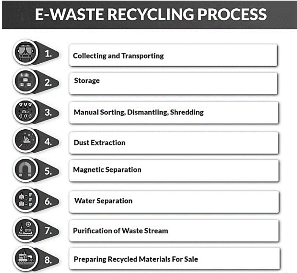
Figure no 4.11 E waste Recycling Procedures
